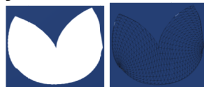
Fig. 10. Curve surface is flattened to plane surface with its meshing structure.
